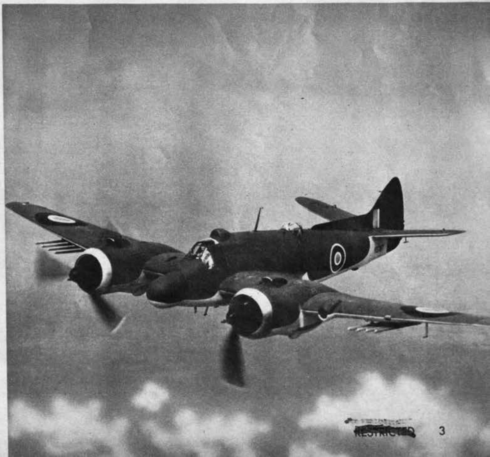
Beaufighter X (above and below) has added a snoutlike radome and a long dorsal fin to its basic airframe, giving it one of the war's most irregular plane shapes. Radome extends the Beau's short nose, while dorsal fin makes recognition easier.
